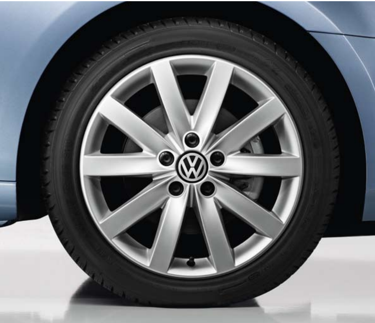
The 6J X 15 'Wellington' alloy wheel with size 195/65 R15 tyre highlights the reliability of the New Golf. Standard on the Trendline models.
