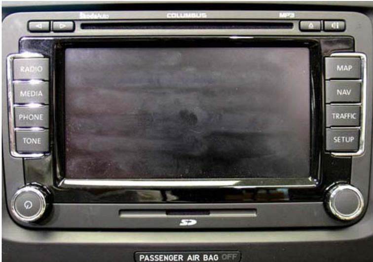
10. After 5 minutes without any activity, it is necessary to switch on the RNS using the bottom round button (left side); restart the navigation before bringing the device into emergency mode; the restart is carried out by pressing both buttons on the left side (arrow to the left and to the right) and one of the two buttons on the right side with the loudspeaker and microphone symbol.
