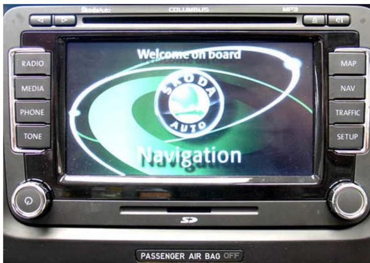
2. Before carrying out the device SW update, restart the navigation. Press both buttons on the left side (arrow to the left and to the right) and one of the buttons on the right side with the microphone symbol.
